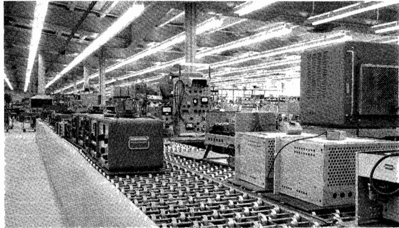
As in Palo Alto, the plant makes extensive use of skate conveyor to speed the production, testing, and shipment of instruments.
